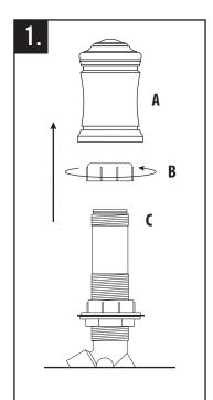
Pull air gap (A) off of upper cap nut
